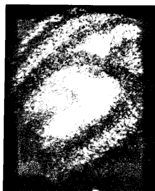
Fig. 2. Interference fringes given by insertion of light diffuser in the path of incident beam.
