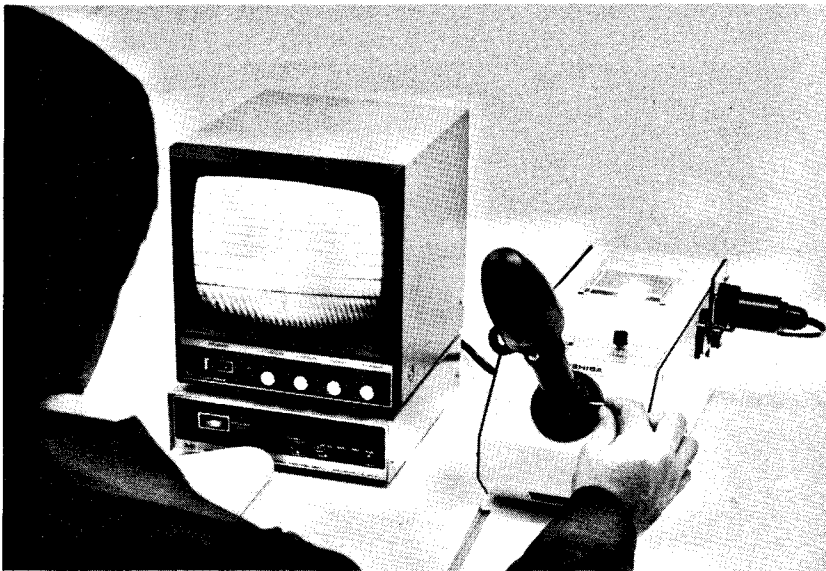
Fig. 9. FSM-10, surface stress meters, for small-size flat chemically tempered glass sheets (right), and equipped with a video display system (left).
